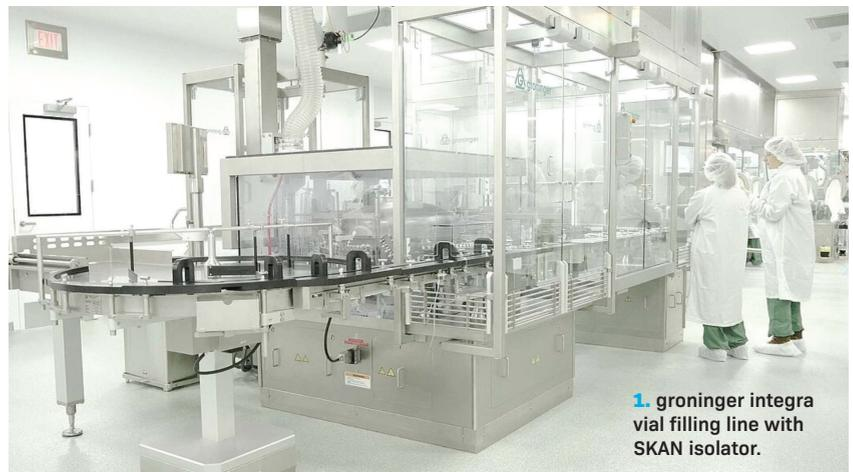
**1. groninger integra vial filling line with SKAN isolator.**
