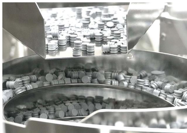
5. The stoppering station uses a vibratory bowl that does not need to be changed for stoppers.
