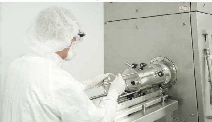
Docking a Beta Canister on an MTI (Material Transfer Isolator) from SKAN
