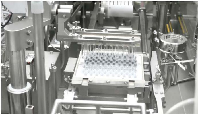
Cartridge in process control (weight check) on a Groninger line
