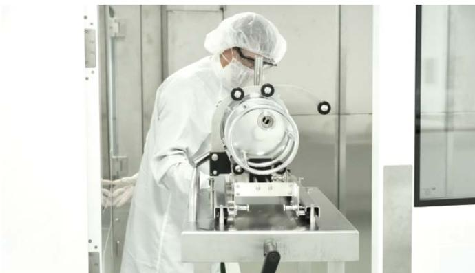
Docking a Beta Canister on an MTI (Material Transfer Isolator) from SKAN2
