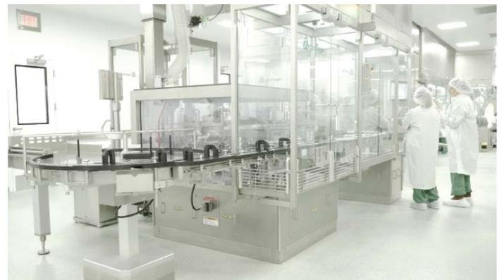
Groninger vial filling line with SKAN isolator, branded integra
